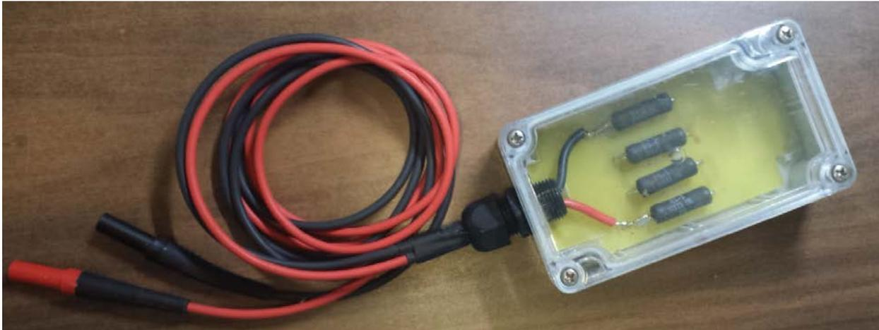
*Figure 1 - Fixed Resistor Box*
